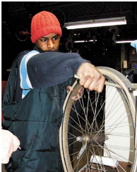
Jake removes a tire tube as he begins work on another bike.
